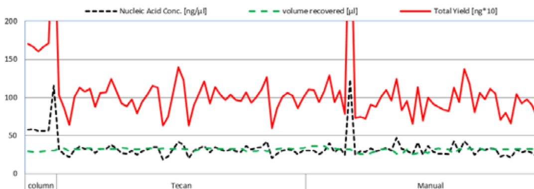
Comparison between manual and automated processing. Data shows concentration, recovery volume and total yield for samples processed across a 96-well plate as well as on single spin columns. Half of the plate samples were processed manually, the other half was processed using the Tecan – Freedom EVO®. Plasmid DNA was purified from E. coli cells grown at 37°C overnight.
