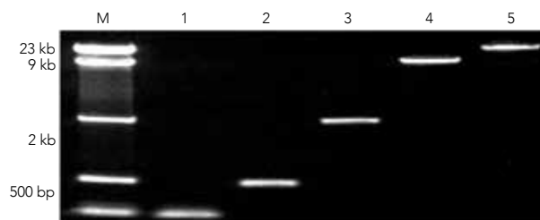
DNA fragments recovered from an agarose gel using the Zymoclean™ Gel DNA Recovery Kit. Lanes: M: DNA Ladder; 1-5: individual ladder DNA fragments.
