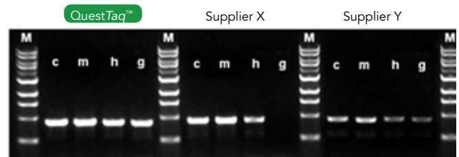
QuestTaq™ consistently yields robust amplicons from DNA templates having modified/unmodified cytosines. The figure shows the level (intensity) of an ~900 bp product generated from DNA templates using QuestTaq™ PreMix and the polymerases from Suppliers X and Y. Lanes correspond to amplicons from template DNA containing: unmodified cytosine (c), 5-methylcytosine (m), 5-hydroxymethylcytosine (h), or glucosyl-5-hydroxymethylcytosine (g). (M) is a 1 kb DNA Marker.
