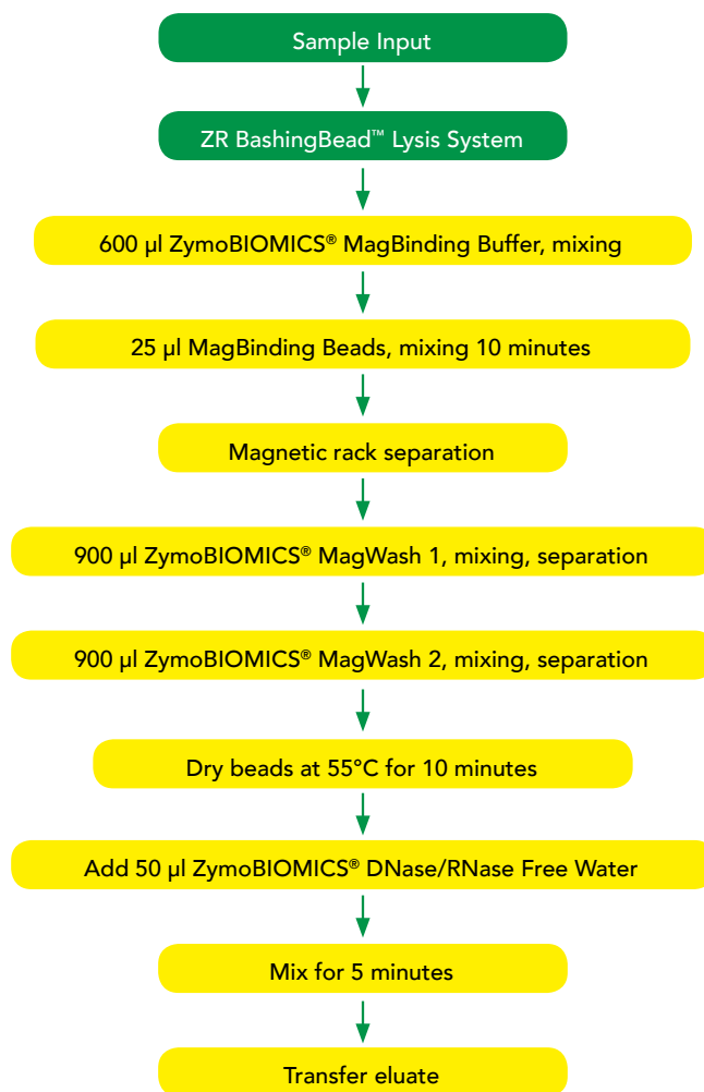
Figure 1. Workflow for the ZymoBIOMICS® 96 MagBead DNA Kit.
